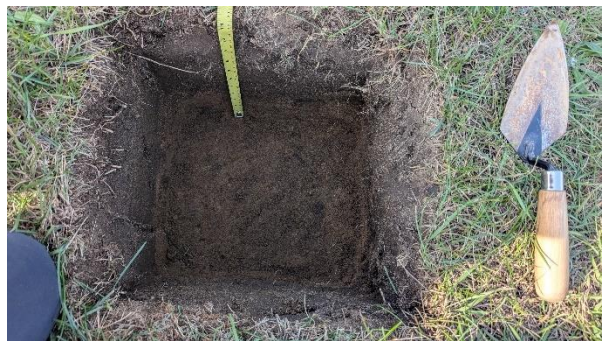
Image 6: Typical test pit.
