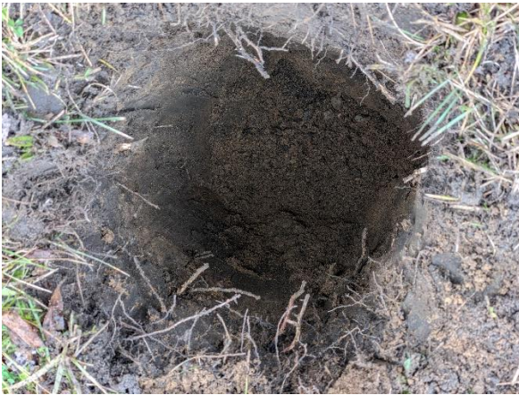
Image 15: Typical disturbed test pit.
